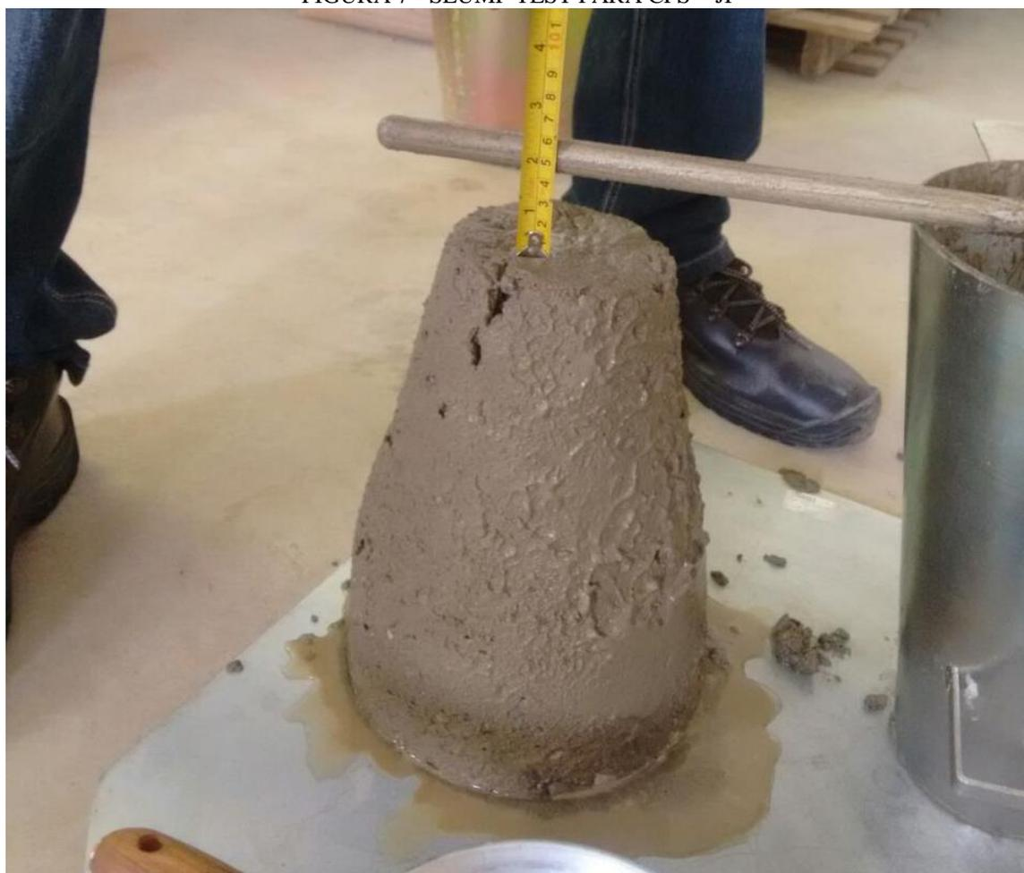
FIGURA 8 - SLUMP TEST PARA CPS – JSP
