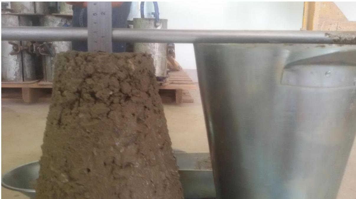
FIGURA 7 - SLUMP TEST PARA CPS – JP
